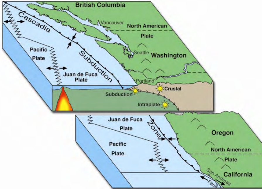
Figure 37. General Source Areas for Subduction Zone, Crustal Earthquakes, and Intraplate Earthquakes
