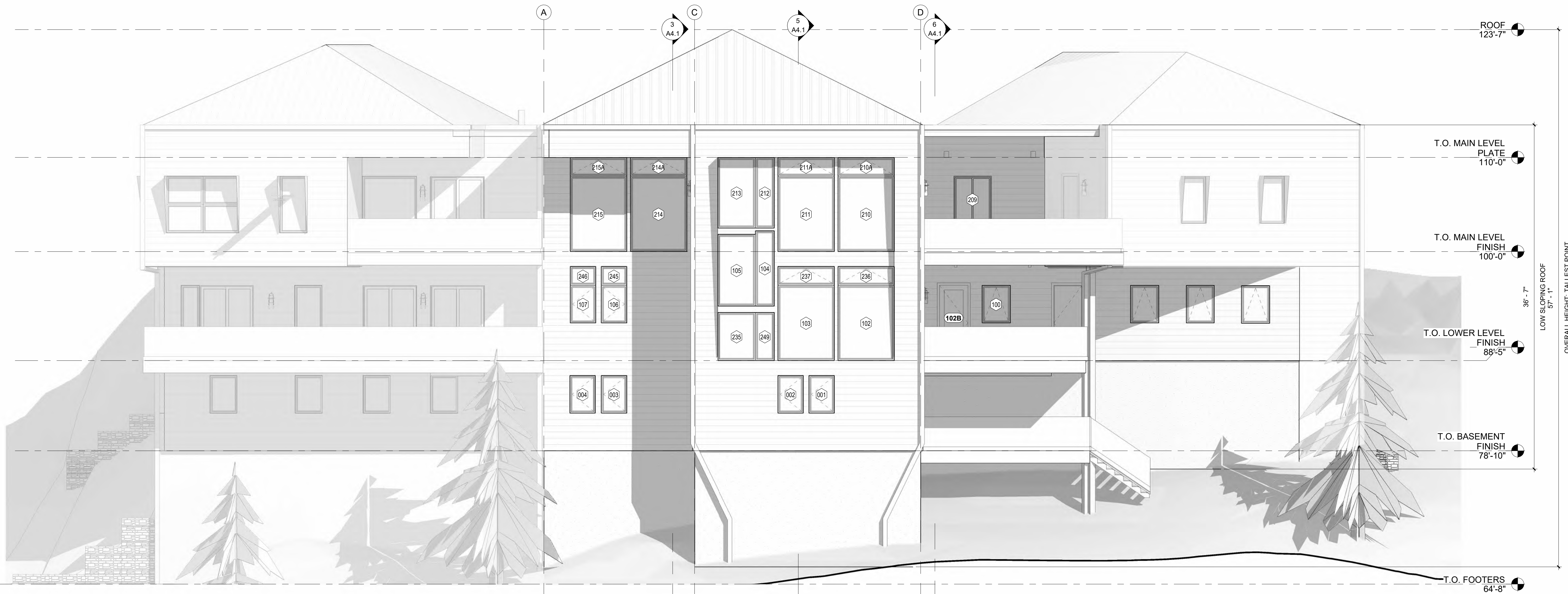
2 OVERALL BUILDING ELEVATION - WEST 3/16" = 1'-0"
