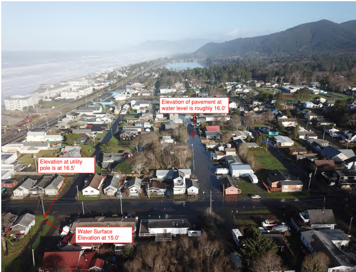
Figure 7 – Water Surface Elevation During Flooding
