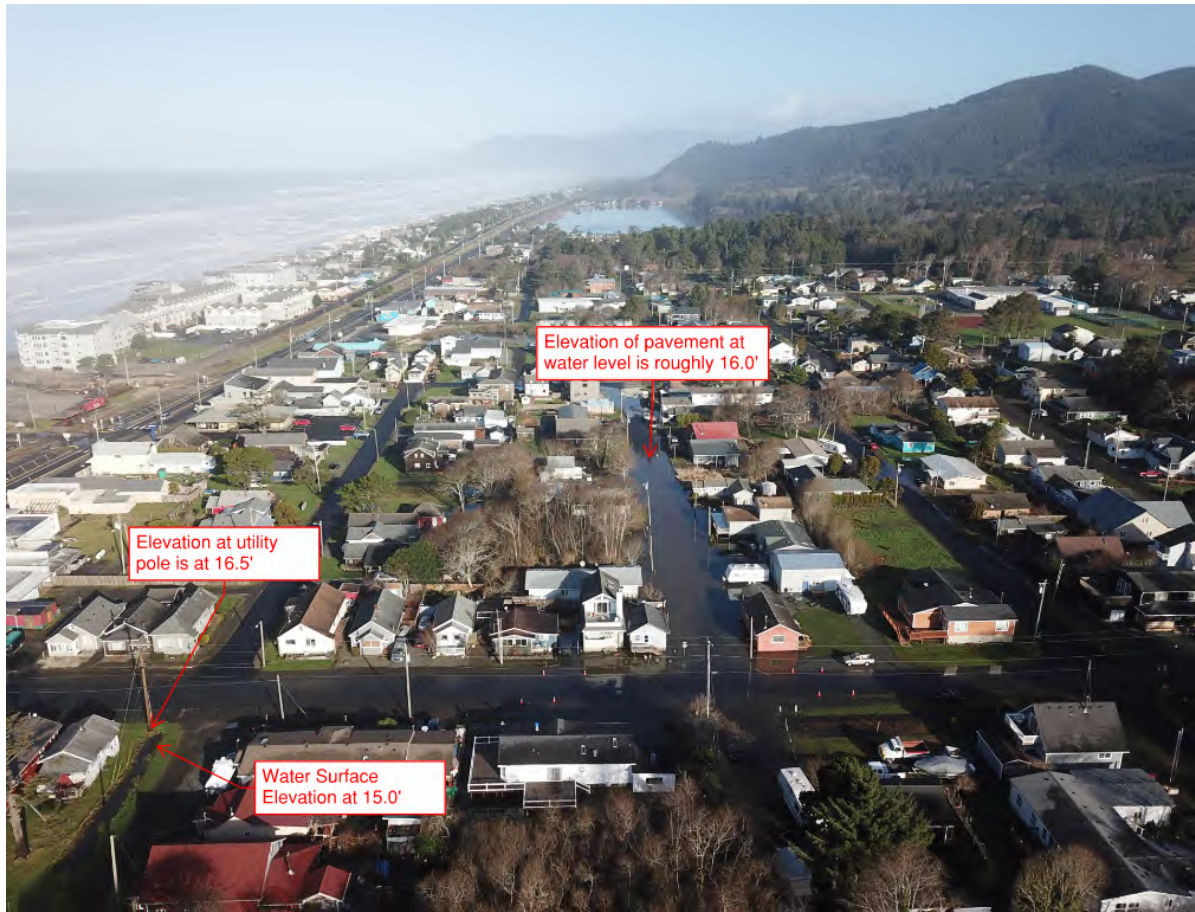
Figure 7 – Water Surface Elevation During Flooding
